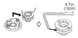
4. Wind up the line in the correct direction as indicated on the spool.
